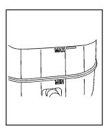
The fluid level should be above MIN. If it is not. have your brake hydraulic system checked to see if there is a leak.
